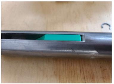
4. The next part is important to make sure that you are careful. When the pin from the ram is removed, the ram can fall, make sure you foot is not under the ram. Remove the C-Clamp ring that goes around the pin on the ram.
