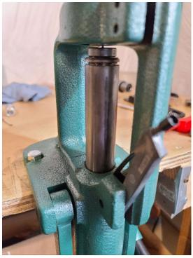
9. Installing the primer catcher can be a bit tricky, mostly because I made it very tight once installed to help prevent slop and movement. You should be able to install it with your left hand only. Insert the bottom slot into the groove on the press. And the with your left hand, press firmly against the bottom left of the primer catcher. It should snap the right side into place.
