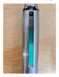
3. Make sure the wedge is flush or recessed slightly into the ram slot so that it will not rub when the ram moves.
