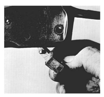
After the screws are removed, move the carrier toward the rear, and take it out downward. Note that the carrier plunger may jump into one of the screw holes during removal, and a drift punch will then have to be inserted to depress the plunger and free it.
