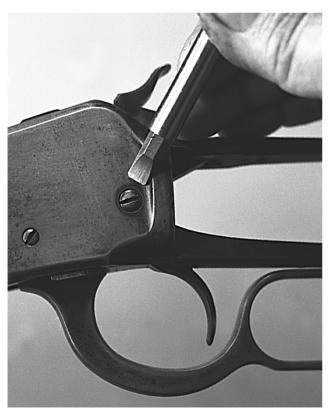
Partially open the lever to give access to the hammer spring screw and strain screw, at the rear of the lower tang. Loosening the strain screw will make removal of the spring screw easier, but this is not absolutely necessary. After removal of the spring screw, disengage the spring hooks from the hammer stirrup, and take out the hammer spring toward the rear.
