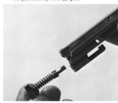
When replacing the lever and its bolt connector pin, once again insert a locking block from below, to hold the bolt in full forward position during replacement of the pin. Also, note that the pin is beveled on one end, and this end should be inserted.
