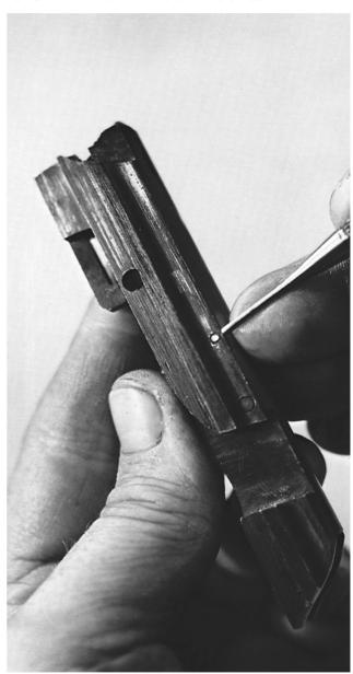
Drift out the larger of the two cross pins in the bolt, the firing pin retaining pin, and take out the firing pin toward the rear.
