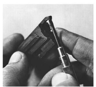
15. After the pin is drifted out, do not lift the extractor upward, as this may break its tempered tail. Hook a small screwdriver under the forward beak of the extractor, and lever it straight out toward the front.
