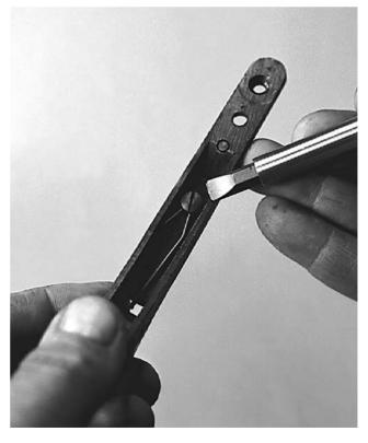
With the lever opened, remove the lock screw in the left locking block, the screw nearest its lower edge.
