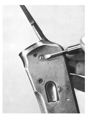
Removal of the cartridge guide screws, one on each side, will release the guides to be taken out of the inside of the receiver. The left guide has the cartridge stop mounted on a vertical pin at its forward end, and the cartridge stop spring is in a recess in the back of the guide. The spring is freed by removal of the guide mounting screw, so take care that it isn't lost during removal of the guide.
