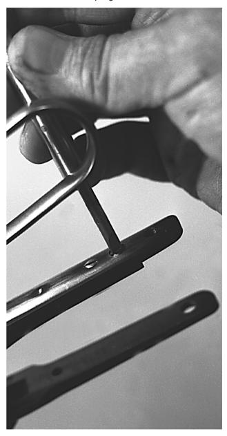
Remove the cross screw on the left side at the rear of the receiver that retains the hammer and the lower tang/trigger housing unit. Pulling the trigger to relieve its spring tension on the hammer will make the removal of the screw easier.
