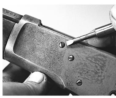
**9** Remove the lever pin cover screw, located on the left side of the receiver at the upper front.
