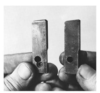
When replacing the locking blocks in the receiver, remember that the one with the lock screw goes on the left side.
