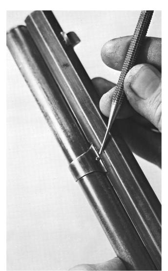
Remove the screws on each side of the forend cap, and move the cap forward along the magazine tube.
