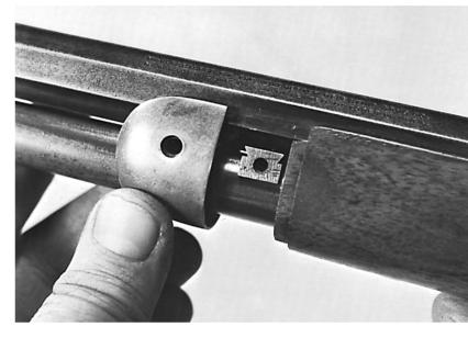
Drift out the small cross pin in the magazine tube hanger loop, and remove the magazine tube toward the front. The forend is now moved forward, the downward and off.
