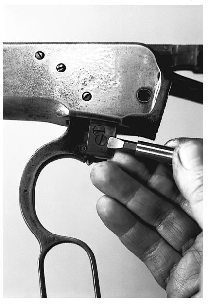
8 The part above the screw, although slotted, is not a screw. It is the cross pin that links the locking blocks to the lever. Push out the cross pin toward the left. Then remove the right and left locking blocks downward.
