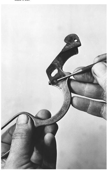
Removal of the lever pin will also have freed the ejector and its collar and spring, and these can now be taken out of the breechblock toward the front.
